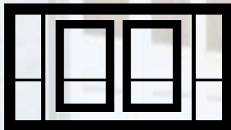
HT3 with 2 mullens positioned to accept 2 x 430 window infill cassettes and 1 x 880 door cassette.
