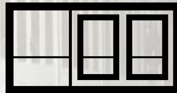
HT3 with 1 Mullen positioned to accept 1 x 880 window cassettes, 1 x 880 door cassette.
